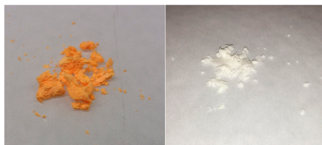
Figure 7. Digital photographs of bulk polymer material before (left) and after (right) the enzymatic reaction.
